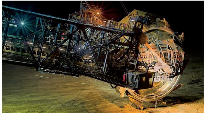
*Highest levels of strain: wear and tear components for bucket-wheel excavators require specific armouring.*
